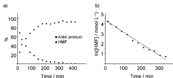
**Figure 4.** Kinetic analysis of aldol condensation between HMF and acetone: a) reaction profile and b) plot of logarithms of HMF concentration versus time for HMF disappearance [373 K,  $\text{MgAl}_2\text{O}_4$ , HMF/catalyst = 1.5 (w/w)].
