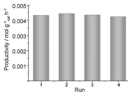
Figure 7. Reusability of the MgAl<sub>2</sub>O<sub>4</sub> catalyst at 373 K.
