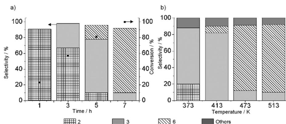
Figure 8. Hydrogenation of aldol product 1 over Cu/MgAl<sub>2</sub>O<sub>4</sub> a) at 473 K at different time intervals and b) at different temperatures for 7 h reaction time allowing full conversion.
