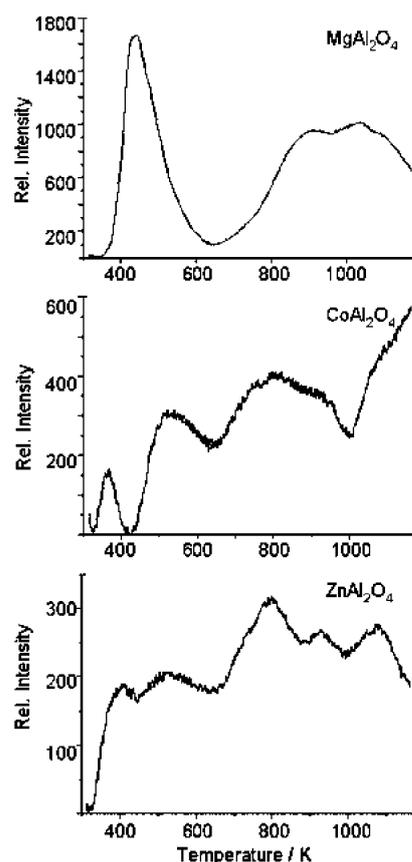
Figure 6. CO<sub>2</sub>-TPD spectra of a) MgAl<sub>2</sub>O<sub>4</sub>, b) CoAl<sub>2</sub>O<sub>4</sub>, and c) ZnAl<sub>2</sub>O<sub>4</sub>.
