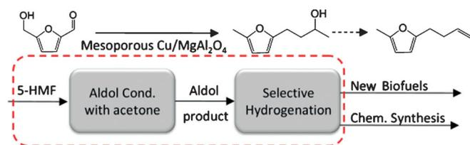
**Scheme 1.** Reaction steps catalyzed by Cu/MgAl<sub>2</sub>O<sub>4</sub>, including aldol condensation of HMF with acetone and subsequent hydrogenation.
